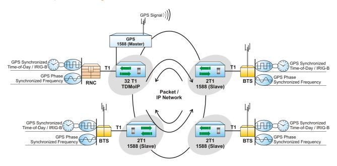
TDM over IP/Ethernet: Using IEEE 1588v2\* to distribute T1s, ToD (Time-Of-Day) and Frequency Synchronization over a Complex Ring and Spoke Optical Fiber Networks
