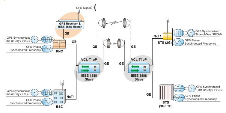
TDM over IP/Ethernet - Distributing T1s, ToD (Time-Of-Day) and Frequency Synchronization over an IP Cloud using IEEE 1588v2\*
