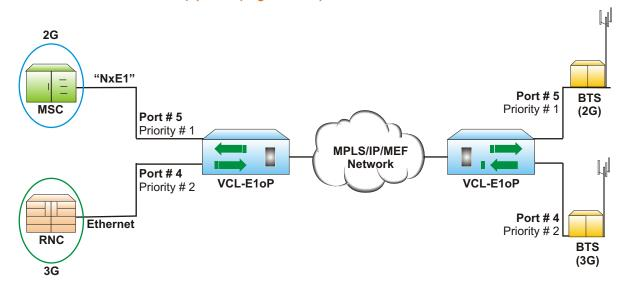
**Notes:** Port based Priority feature allows the user to assign priority to the 2G and 3G traffic ports, so that traffic can be regulated according to the port on which that service is connected.
