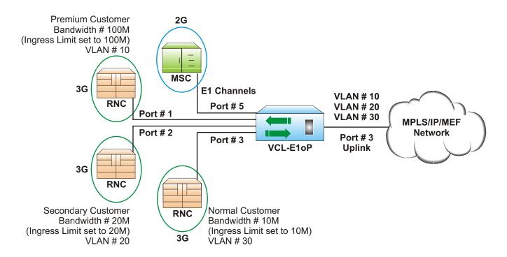
**Notes:** Port based Ingress Ethernet Rate Limiting allows the service provider to assigned the bandwidth as per customer requirements and separating their traffic by assigning 802.1Q based VLANs.
