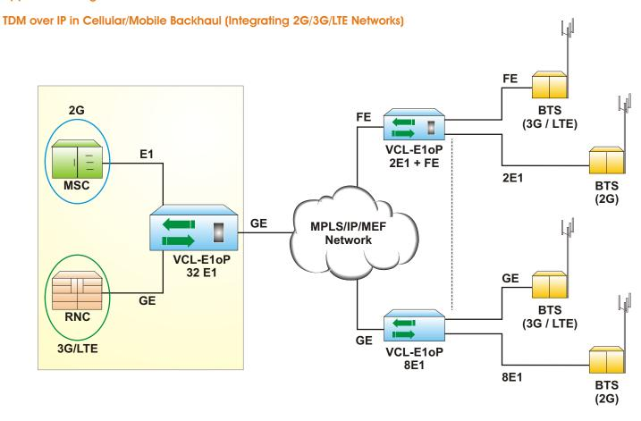
TDM over IP for 2G/3G/LTE - Typical Application in a redundant Wireless Network (1+1 Link Redundancy)
