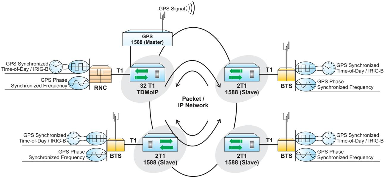
TDM over IP/Ethernet: Using IEEE 1588v2\* to distribute T1s, ToD (Time-Of-Day) and Frequency Synchronization over a Complex Ring and Spoke Optical Fiber Networks
