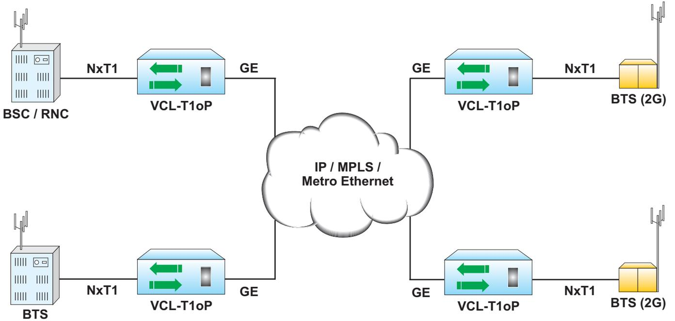
**Note:** Application illustrates link protection using Spanning Tree Protocol between all nodes.
