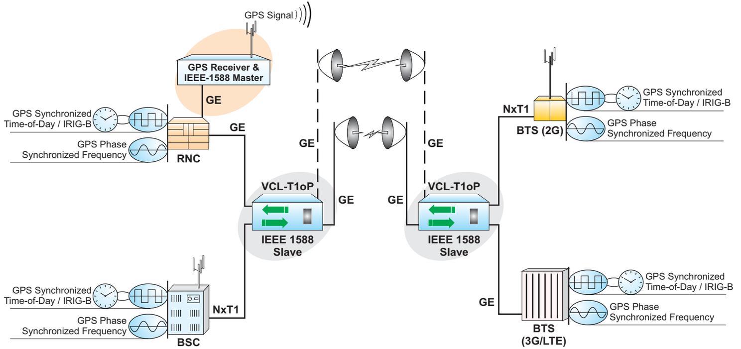
TDM over IP/Ethernet - Distributing T1s, ToD (Time-Of-Day) and Frequency Synchronization over an IP Cloud using IEEE 1588v2\*
