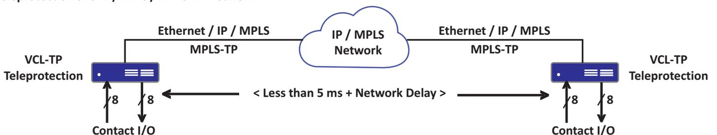
Transmission interface provides both, Ethernet/ IP/ MPLS, 10/100BaseT (Electrical) and 100BaseFX (Optical) Ethernet transmission interface options.
