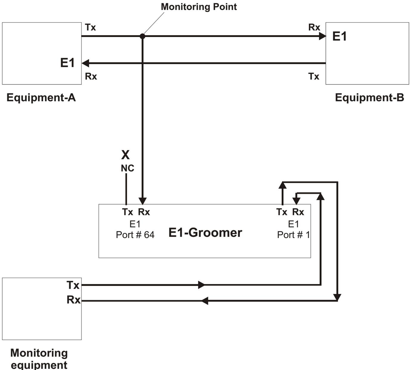
To monitor an E1 link in a single direction, you will need to connect one high impedance E1, RX pair of the Groomer, as it is only the Rx (**Receive**) pair that is capable of listening. Please leave the Tx (**Transmit**) pair un-connected.
