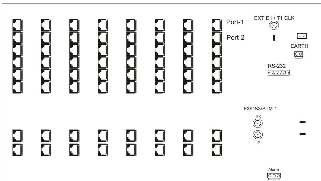
64 Port E1 VCL-MegaConnect Groomer offers programming via an RS232 port for control and monitoring of the unit.
