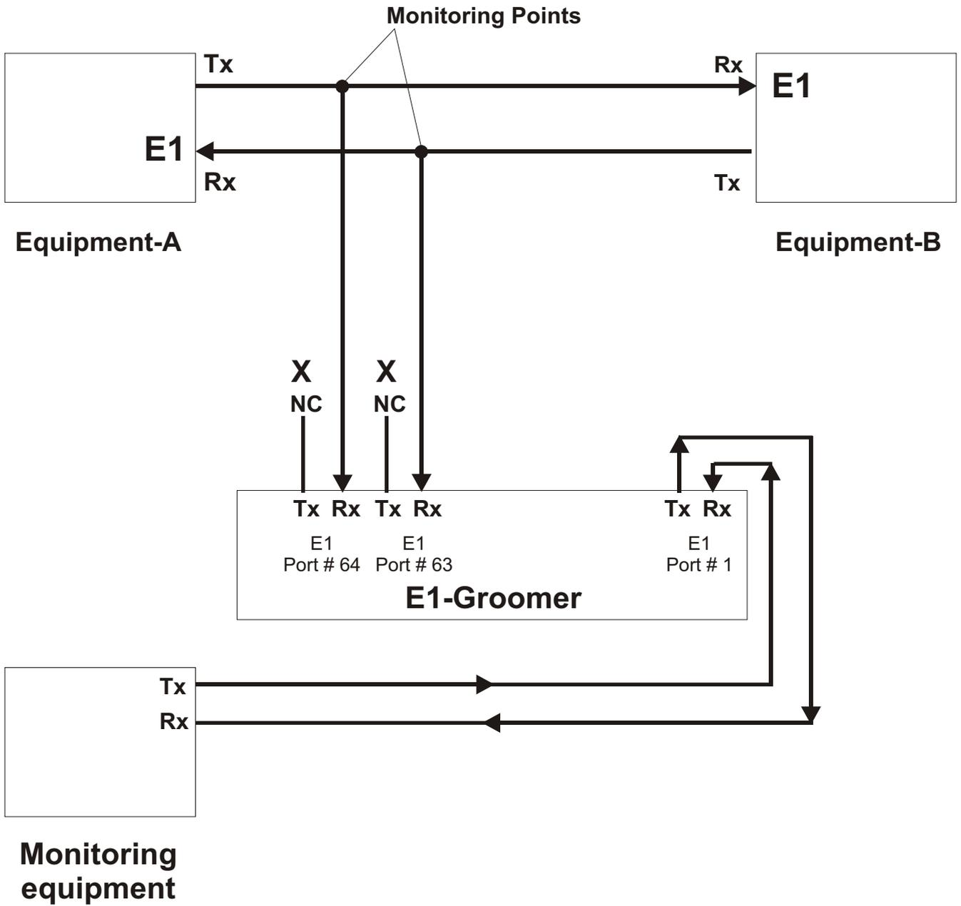
To monitor an E1 link in both directions, you will need to connect two high impedance E1, RX pairs of the Groomer, i.e. use 1, Hi-Z E1 ports.
